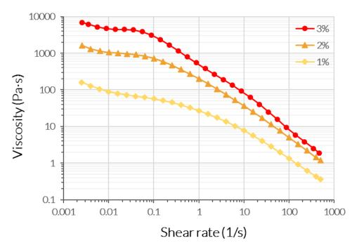
Figure 1. Viscosity of CELLINK Glucomannan dissolved in PBS at different concentrations over a shear rate range of 0.002 to 500 s<sup>-1</sup>, 25°C.
