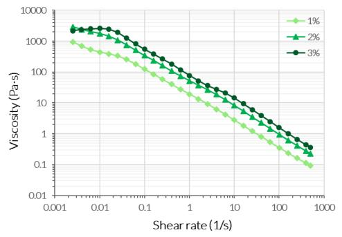
**Figure 1.** Viscosity of CELLINK Xanthan Gum dissolved in PBS at different concentrations over a shear rate range of 0.002 to  $500 \, \text{s}^{-1}$ ,  $25 \, ^{\circ}\text{C}$ .
